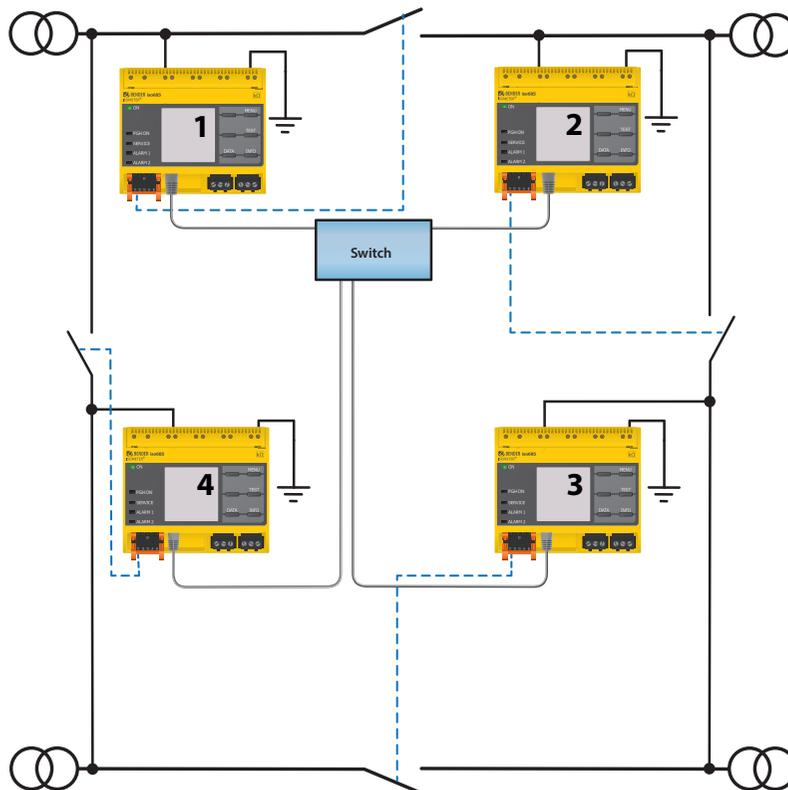
The measuring device with the lowest BCOM address in a team (in the example, device 1) distributes its currently measured insulation value to all team members (here device 2). The parameter "Measured value subscription" can be used to define whether this shared measured value is to be shown on the respective device. If this function is activated, device 2 would also report an insulation alarm 1 and 2 based on the selected alarm thresholds. This function is activated by default.
