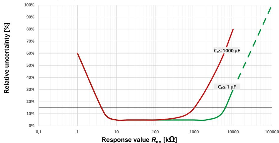
Percentage relative uncertainty as a function of the response value and system leakage capacitance according to IEC 61557-8 ( $U_n = 690\text{ V}$ ,  $f = 50\text{ Hz}$ ) measuring range  $> 10\text{ M}\Omega$
