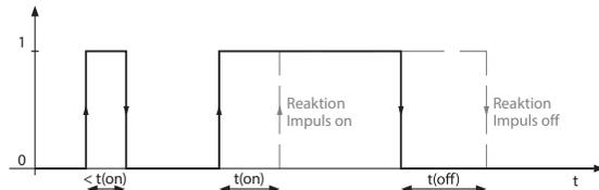
**\*Active low** An event is carried out on the falling edge of the digital input (high to low). Response time  $t(\text{on})/t(\text{off})$  after a switch-off signal.
