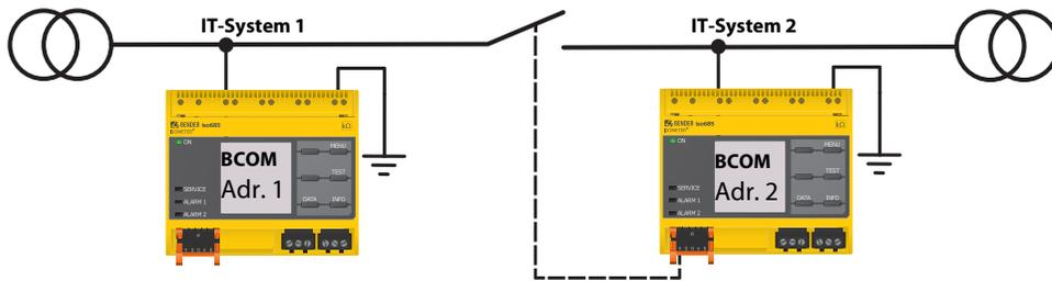
Via the X1 connector, the ISOMETER® can be isolated from the IT system and the measuring functions can be deactivated. Therefore, the function of the digital input in use has to be set to "Device inactive".
