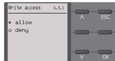
Factory-set to "Deny". A parameter change via the web server is only possible if you allow write access in the device.
