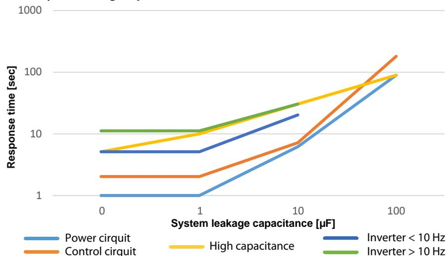
Typical response times for DC alarm for RF depending on system profile and system leakage capacitance (isoHR685W-x-I-B)
