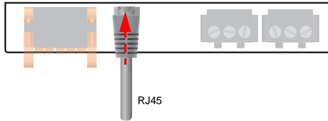
Connection with standard patch cable (RJ45/no crossover cable) to other ISOMETER®s or interconnection of several ISOMETER®s in STAR topology via a switch.
