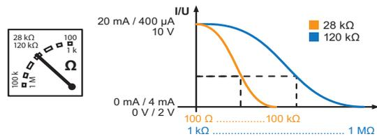
Calculation of the insulation resistance using the analogue output:
